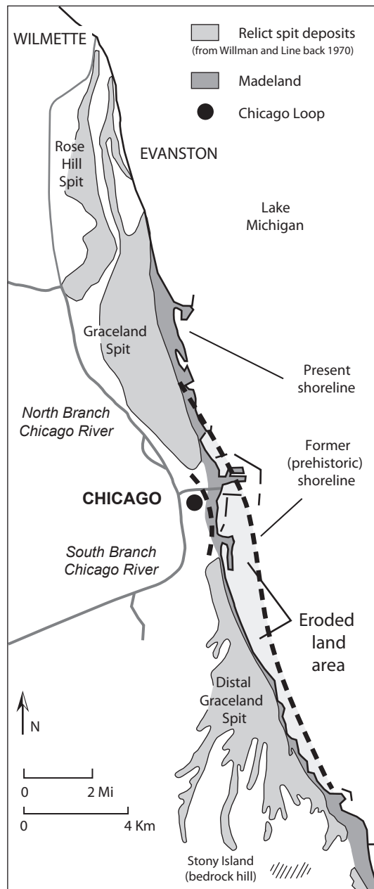
Figure 4-1. The present central and south Chicago lakefront previously had a shoreline farther lakeward than the present-day madeland shoreline. This is demonstrated by the Graceland spit which is preserved north and south of the Chicago Loop but is absent in the Loop vicinity. The erosion of the former land area occurred within the past 2,500 years and was likely in progress at the time of early settlement at Chicago (modified from Chrzastowski 2005).
